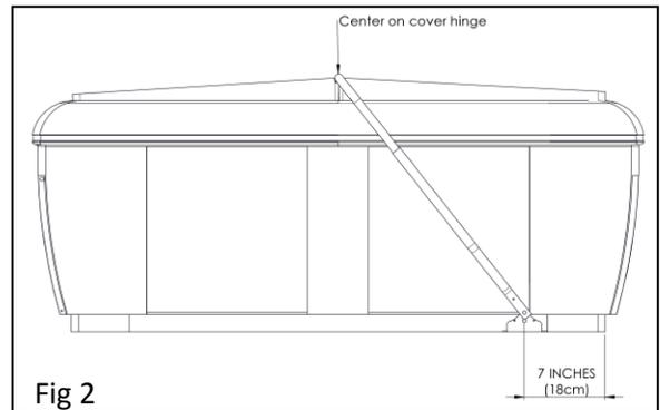
3. While lifting the tube connected to the base bracket, slide the short end of a support tube into the base bracket tube. Rest the long end of the support tube on the center of the cover hinge.
